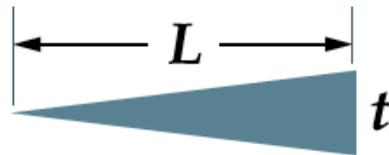
A wedge is a movable double incline plane used to separate objects by the use of force. Examples include a knife, ax, and nail.
