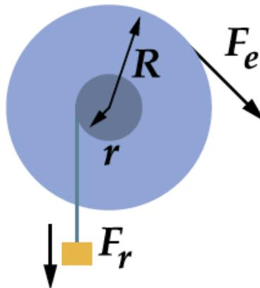
A wheel and axle is essentially a modified lever, but it can move a load farther than a lever can. The center of the axle serves as a fulcrum. Gears, belts, cams, and cranks include applications of a wheel and axle.
