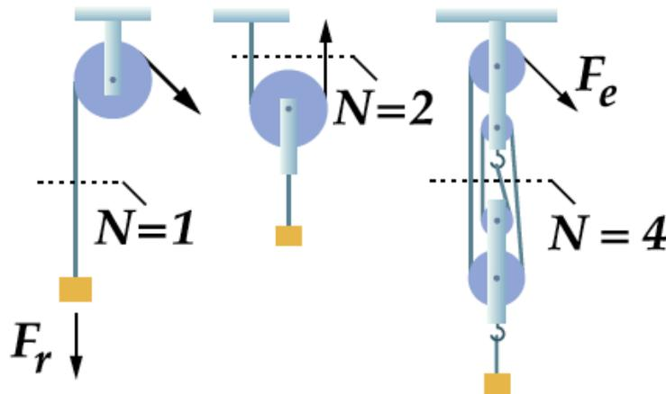
A pulley is a wheel over which a rope or belt is passed. It is also a form of the wheel and axle. Pulleys are often interconnected in order to obtain considerable mechanical advantage. Pulleys may be used to change the direction of the force or to increase the ease of lifting an object.
